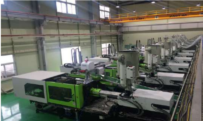
Automated Plastic Injection(13 machine)
